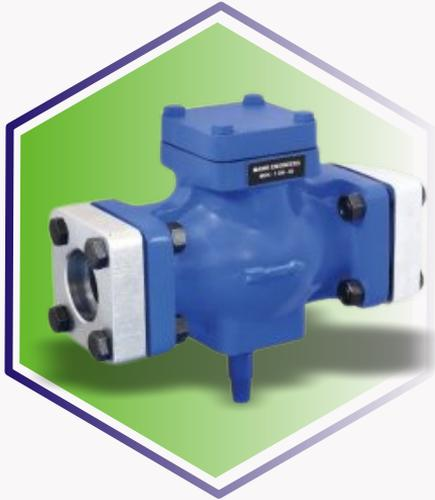
The MCK-1 are flanged, heavy-duty, piston-type check valves control the flow of refrigerant. Valves open wide for flow in the direction of the arrow on the valve body. Valves close tight when flow reversals occur. The piston design minimizes pulsations.
