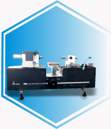
Model: Lab Microcal 600 comes with measuring spindle cross section of size (60x40mm) for rigidity & straightness accuracy < 1 micron. Measuring head carriage precisely preloaded & aligned with special bearing to ensure the lifetime accuracy. Adjustable anvil design ensures parallelism of measuring faces of anvil.
